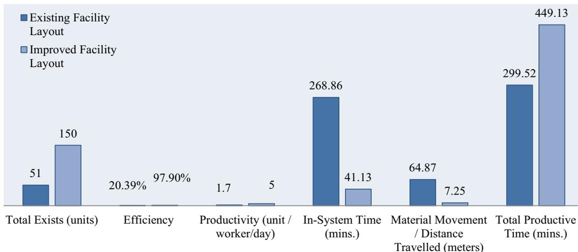
**Fig. 4** Comparison of existing and redesigned facility layout
