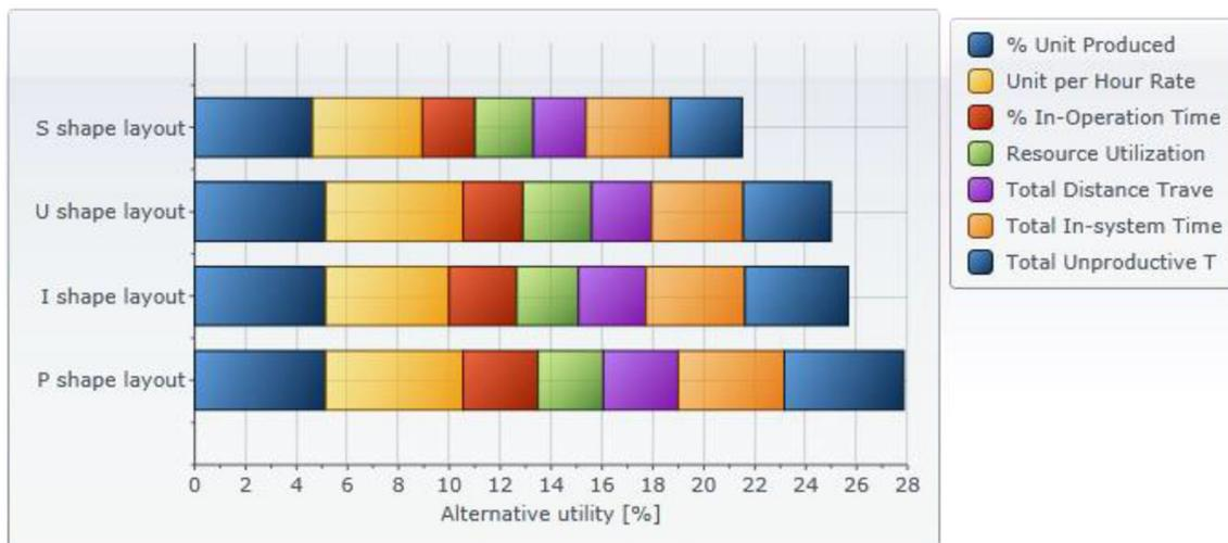
**Fig. 3** AHP result of simulated facility layouts (redesigned)
